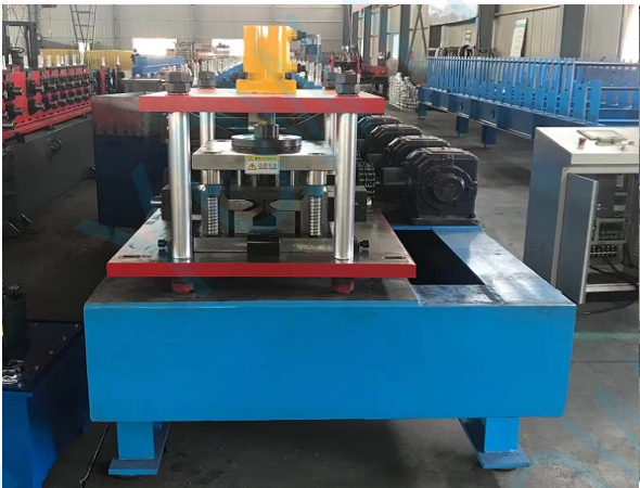
Hydraulic mould cutting
