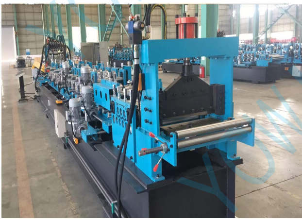
Feeding and hydraulic pre-cutting
