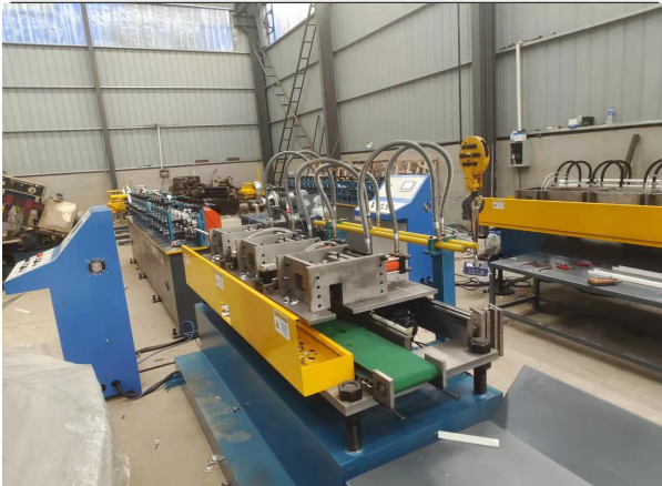
Automatic T ceiling production line
