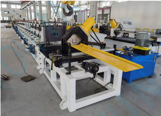
Storage rack hydraulic cutting
