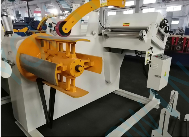
Decoiler with the leveling machine
